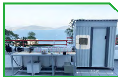
Figure 2: Assembly and operation of the elastocaloric cooling device (Photo credit: Nature Press)
